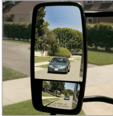
Standard split-view driver and passenger mirrors help eliminate blind spots
