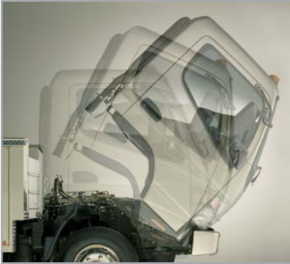
Cab tilts forward for easy servicing
